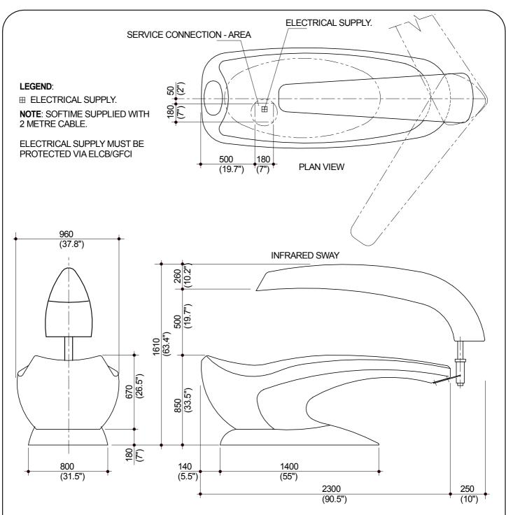
NOTE: MAIN BODY, SEPERATES FROM BASE, INFRA-RED SWAY REMOVES FROM BRACKET. TO ALLOW ACCESS THROUGH STANDARD DOOR OPENING
